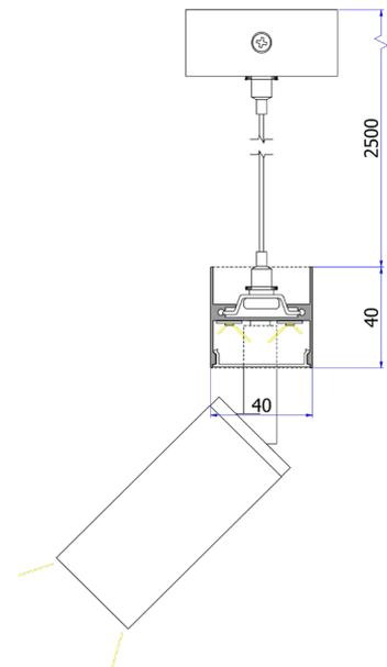
**EVO1 - PERFIL PENDENTE COM CABO + SPOTS FOCUS MINI MR11 GU10 - 2000 x 40 x 40 mm**
